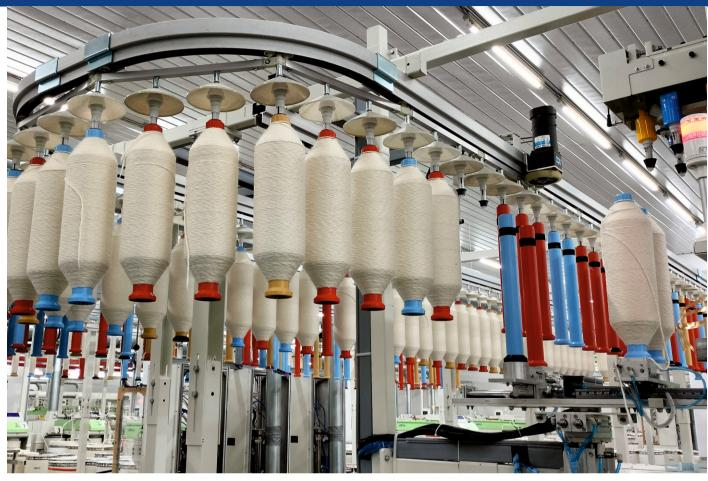
We are the manufacturer and global supplier of fully automatic roving transport system for LMW OEM & retrofit machines. It transports the Full Bobbins from Speed Frame to Ring frame machines and the empties back to speed frame machines just by a push of button.
