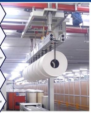
Lap formers are connected to comber through Lap transport system. Upon request from a comber nearing exhaust of the running laps, Full laps (8 Nos.) are transported through LTS to the respective comber. Then the empty spools from the comber moved back to Lap former automatically. The lap transport system enhances the efficiency of combing machines and reduces the labour cost.
